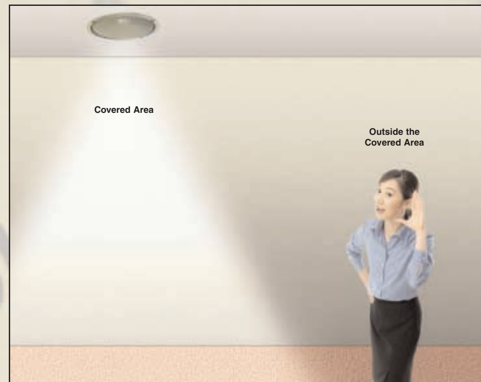
Figure 6 A loudspeaker will sound quite different as you change your listening position
