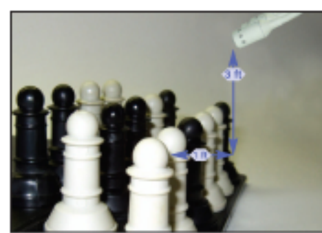
Figure 7 Position the microphone one foot in front and three feet above the front row
